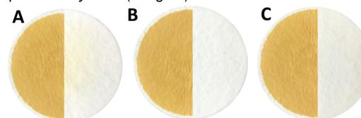
Image 1: Cambridge filter pad showing particulate matter collected for (A) THP aerosol (B) HYB aerosol and (C) *myblu*<sup>TM</sup> aerosol compared to 3R4F particulate emissions
